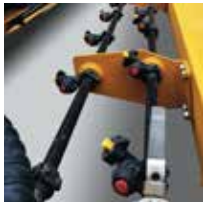
Pressurized Water Spray
