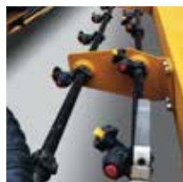
Pressurized Water Spray
